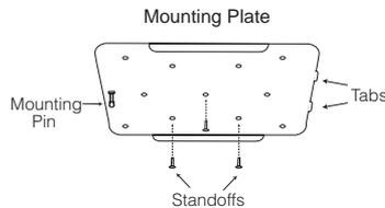
2. Align the HS-DH800 Data/Voice Distribution Hub over the standoffs and snap into place.
